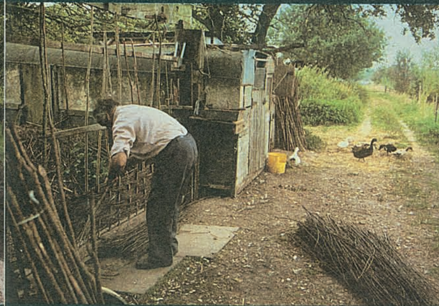
Stan Dare has designed his own frame to weave hurdles from withies—willow branches. He can make six in a day
